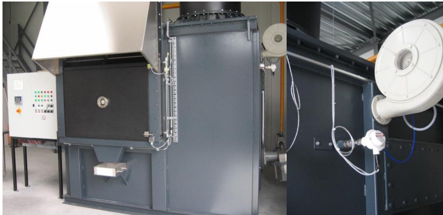
Example of Jongtech incinerator with an Econox HT probe
